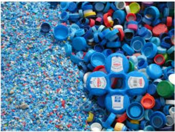
There is a mixture of 70% ground mash with 30% PEHD (high density polyethylene).
